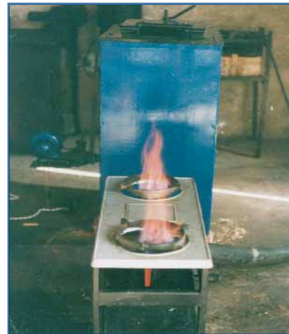
M.H.V. gas generator-stove (China)
