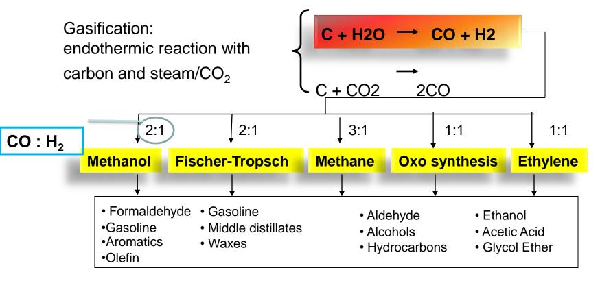
Unfortunately synthesis-gas from wood contains **tars** (mixture of hydrocarbon compounds) and traces of HCI,HF,NH3 and alkaline metals; their concentration depends on the nature of the biomass and the type of reactor. There's also risk of low-melting of ashes. **Tar gas-cleaning can not be considered yet a solved problem !**
